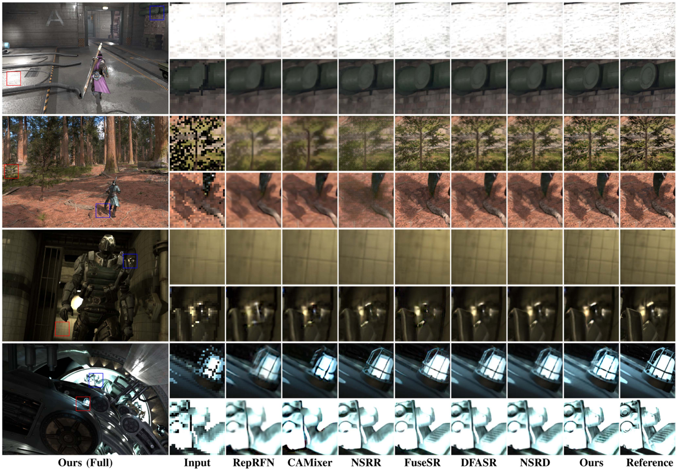
Fig. 6. Visual comparison of different methods for 4 \times 4 upsampling. The results on the BK , RF , SW , and IF scenes are shown from top to bottom. Due to a lack of auxiliary information, RepRFN and CAMixer are unable to recover texture details. NSRR leverages LR G-buffer information, performing better on SW and IF scenes, but its result on the RF scene remains unsatisfying. FuseSR and NSRD achieve higher-quality texture reconstruction with the help of HR G-buffers, but its recovery of strong reflections (1st row of BK ) and shadows (2nd row of RF ) is not accurate. DFASR suffers from aliasing in the tree (1st row of RF ) and the floor (1st row of BK ). In contrast, our reconstructions are realistic, almost on par with the reference images.
