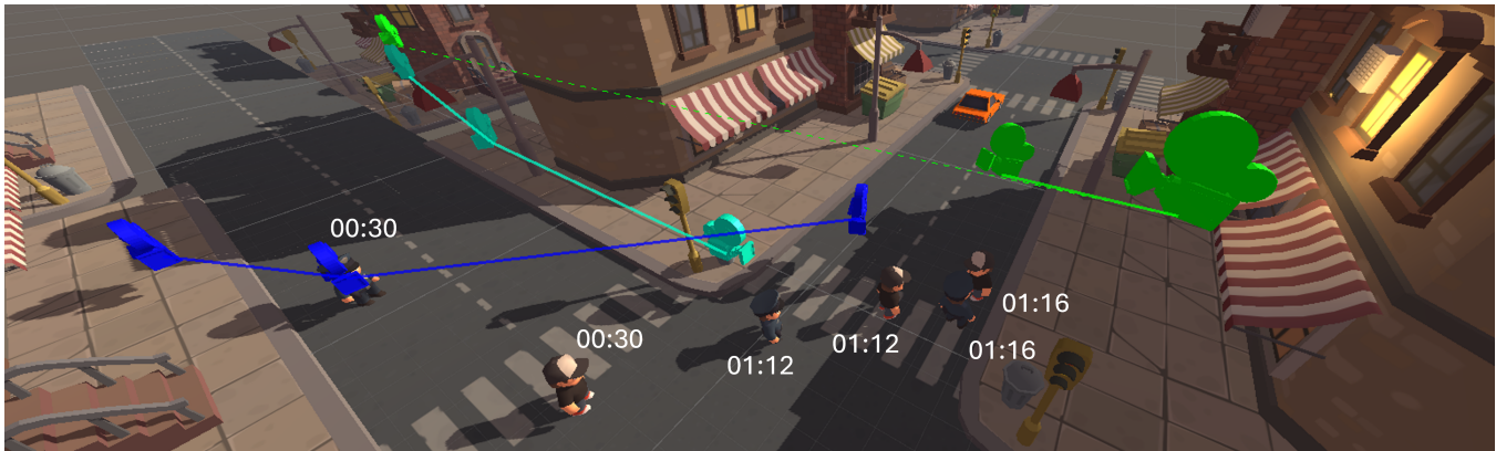
Figure 6: Our deep generative model can generate diverse sequences of camera poses to convey the story of an animation. The three sequences generated for an animation of two characters in this example are visualized as distinct camera trajectories coloured in blue, cyan and green in the 3D scene. Each trajectory consists of three camera poses generated for three keyframes where the two characters belonging to the same keyframe are labelled with their corresponding timestamps. The solid lines on a trajectory indicate the transition of the same camera within a shot and the dashed lines represent the jump between the cameras of different shots.
