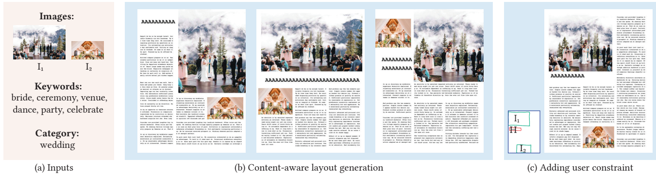
Fig. 1. Our probabilistic generative model can support content-aware layout generation. Given input images, design category, and keywords that summarize the text contents (which are either automatically extracted from the input text or directly provided by the user), as shown in (a), our method automatically generates multiple layouts that fit the visual and textual contents (b). The user may optionally express his/her design intent by roughly sketching some elements on a page, e.g., adding two image elements by sketching two green regions I_1 and I_2 and a headline element by sketching a red region H , as shown in the small diagram in (c). Our method will then generate a layout that matches the user's intent, i.e., two images and a header placed at the specified locations, as shown in the large diagram in (c). The input images are from BRIDES (© Condé Nast).
